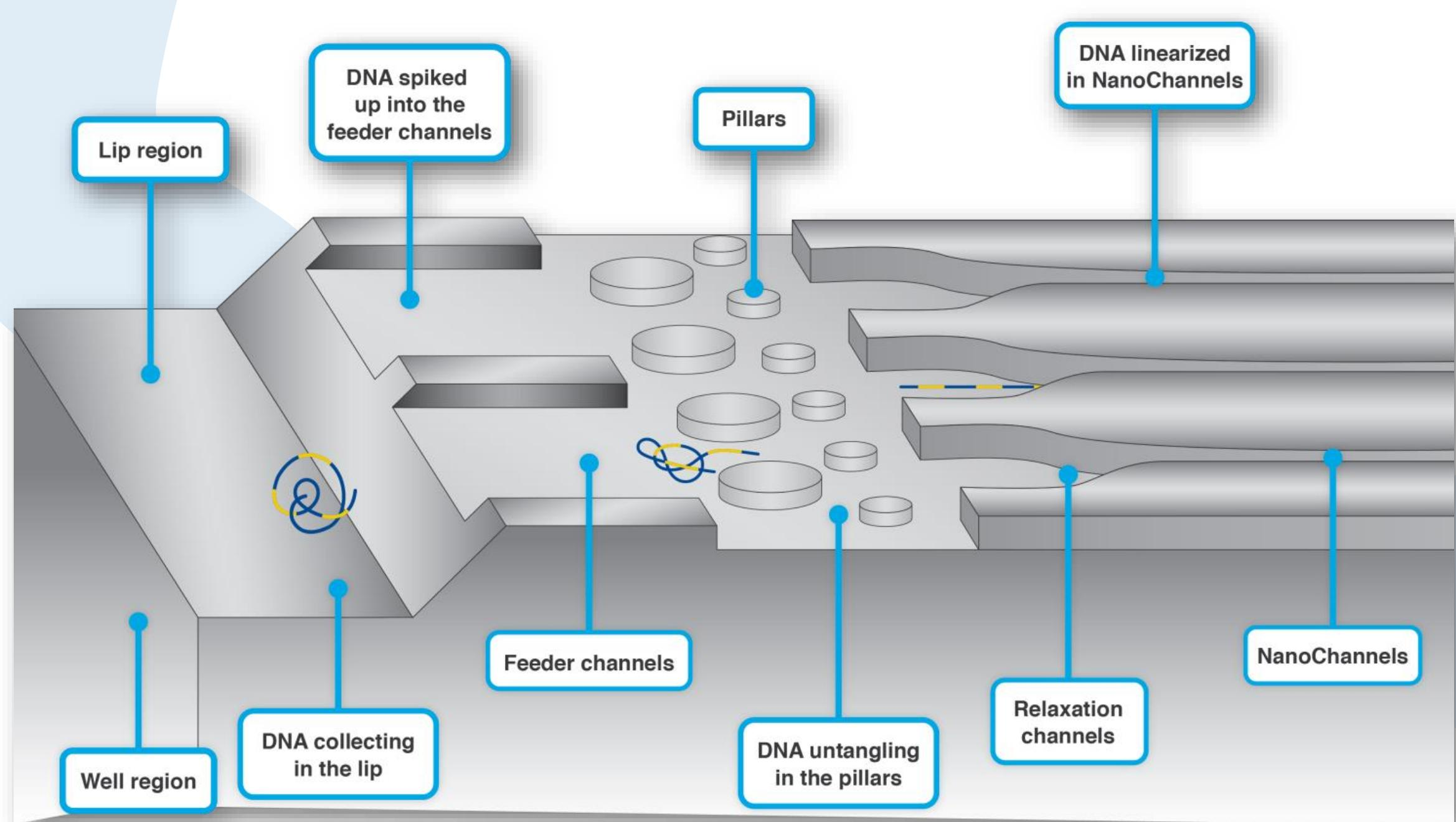
DNA molecules are linearized in the NanoChannels
